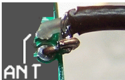
Sample Antenna Connection
